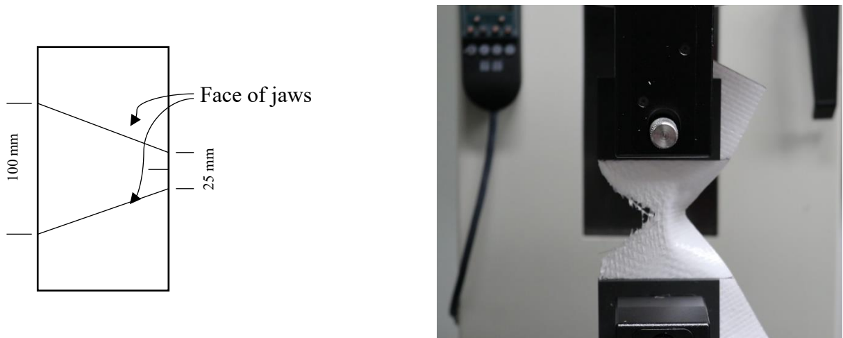
Figure 13: Trapezoid Tear Test schematic diagram and actual test.
