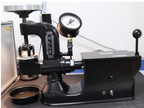
Figure 16: Hydrostatic resistance tester, also by Mullen Testers.
