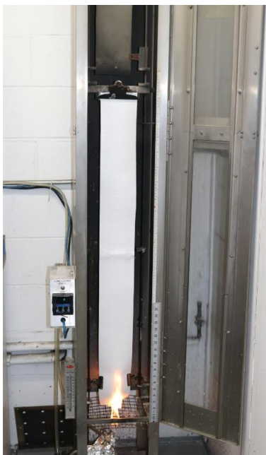
Figure 19: NFPA 701 Method 2 burn test chamber and sample in holder.
