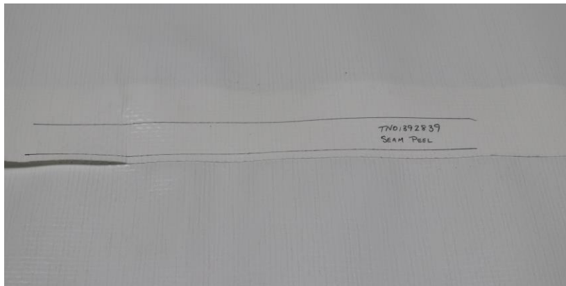
Figure 25: Test specimen drawn on the welded membrane.
