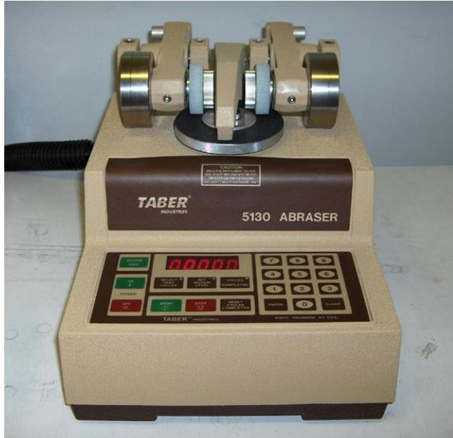
Figure 18: Taber Abraser used to measure the abrasion resistance.
