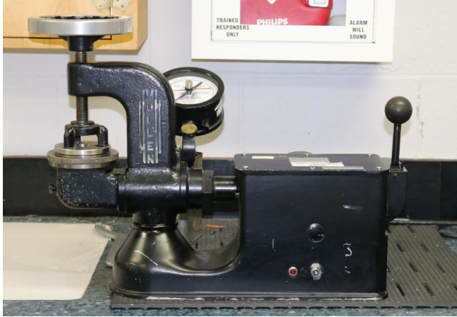
Figure 15: Mullen Burst tester.
