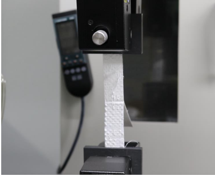
Figure 26: Beginning of seam peel on universal testing machine.
