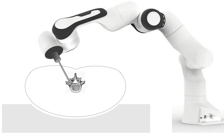
Figure 6.6: Illustration of Franka Emika Panda robot [69] in a minimally invasive treatment on the spine.
