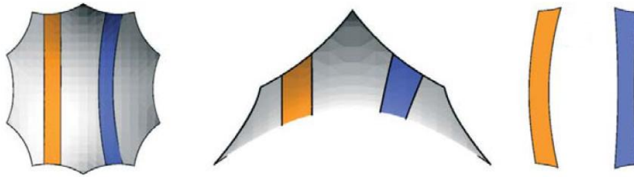
Fig. 9 - Comparison of non-geodesic (orange) and geodesic (blue) cloth generation
