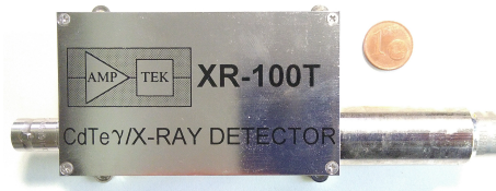
Figure 6.6: Photo of the used semiconductor XR-100CdTe X-ray detector. On the upper right is a 1 cent Euro coin in order to give an impression of the detector size.
