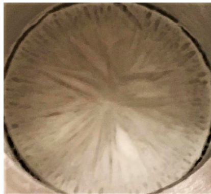
Figure 7. The photograph of the partially dried sample after 11.5 h (top view) reveals a star-like pore structure with long lamellar pores in the center and a rosette with smaller pores at the periphery.
