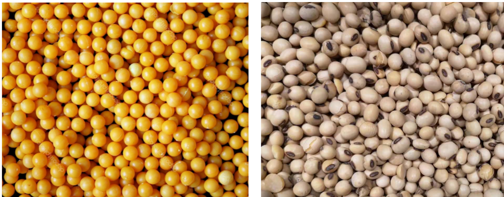
Figure 5.2: Bed materials used in this work: Plastic balls (left) and soybeans (right).
