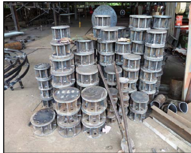
TRUSS FLANGE JOINT
