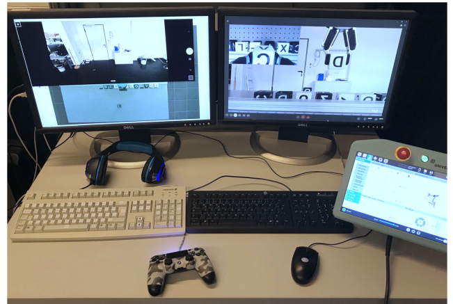
FIGURE 1. Wizard’s chamber: monitors with a handheld controller, UR5e control-panel, one keyboard for shortcuts and another for direct speech output.
