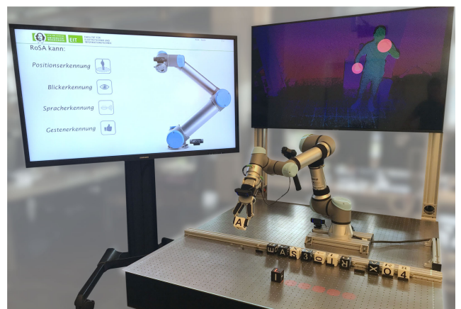
FIGURE 2. RoSA system setup: UR5e industrial robot, “mock-up”-gesture recognition (right), instructions (left).
