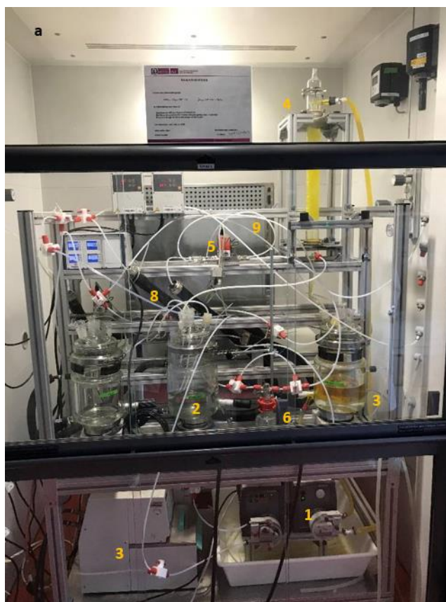
Fig. A.10, Photography of the experimental setup including pumps (1) for supplying the electrolyte stored in vessel (2) to the reactor and the NaOH solution with indigo carmine (by Alfa Aesar) as indicator stored in vessel (3) to the neutralization column (4). The flow rate of gases is controlled by 2 MFCs (5) and the oxygen feed stream is humidified by a gas bubbler (6). The thermostat (7) and the heating tubes (8) around the feed gas tubes allow for controlling the temperature of the electrolyte and the reactor feed gases respectively. The reactor is placed in the oven (9) on the back of the picture.
