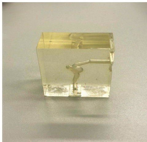
FIGURE 3.13: Silicon cuboid phantom used for the image reconstruction
