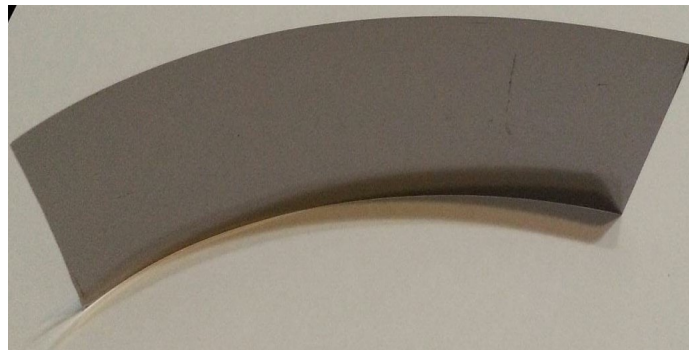
FIGURE 3.15: Tantalum sheet phantom used for image reconstruction
