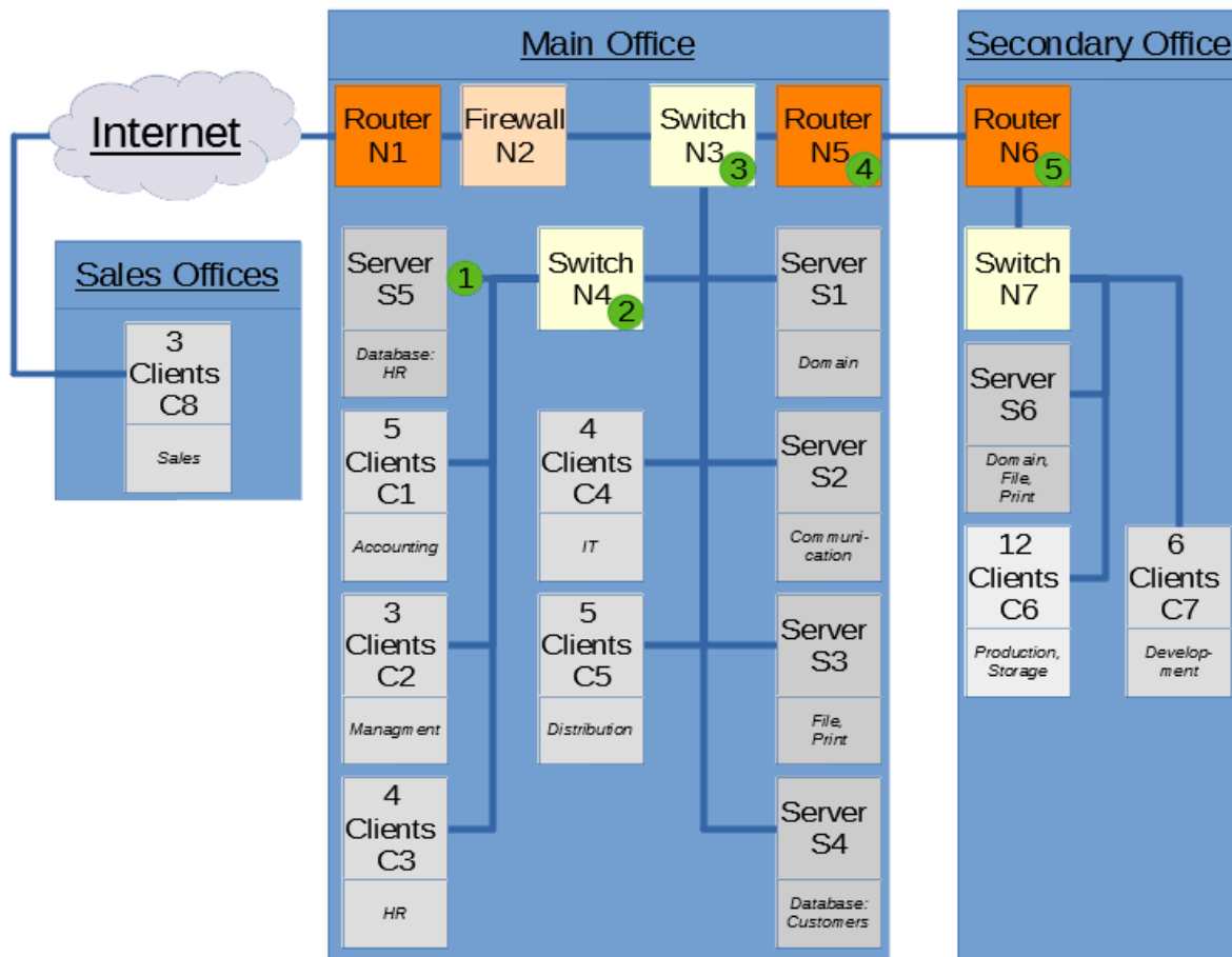
Figure 4.6: Model infrastructure for a small business based on [BSI11] including different potential locations to perform DG
