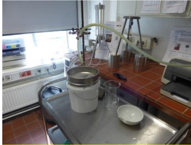
Fig. 2.8 Initiated Water Jet Sieving Setup
