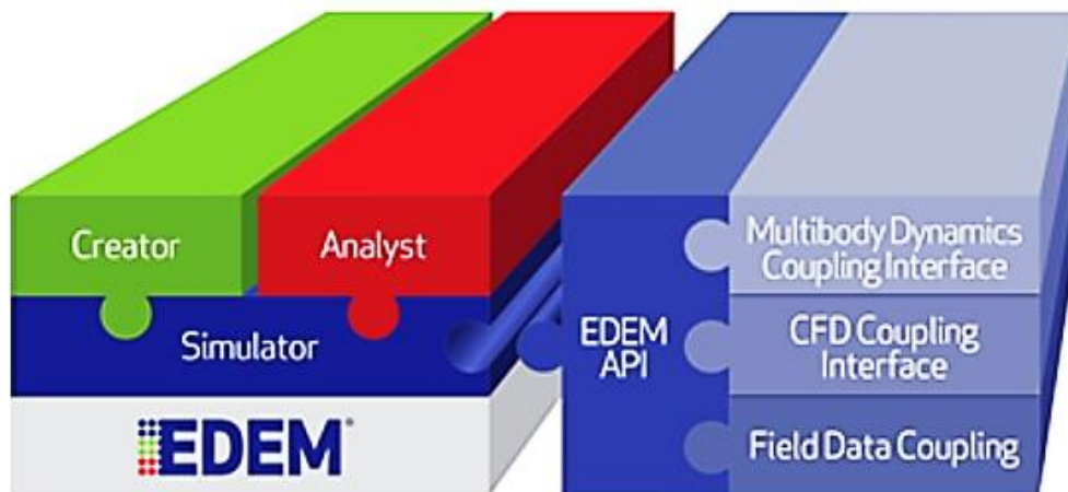
Fig. 6.1 A schematic of EDEM structure and its possibilities for coupling with other modules (see https://www.edemsimulation.com ).
