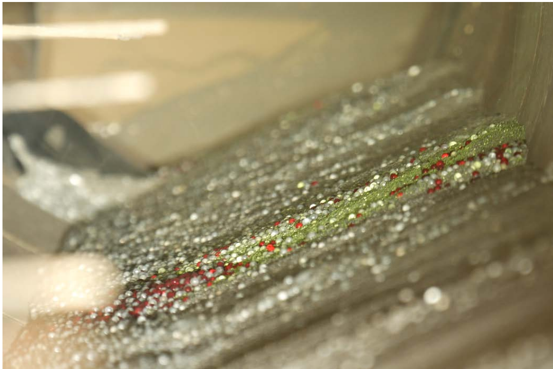
Figure 3.15 Particle bed of 0.7&4 mm mixing particles
