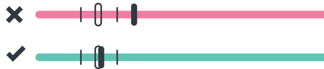
Figure 6.13: Visual feedback for the user for the manual task. The bold line indicates the current position of the input device, the thin lines represent tolerance range and center of the target position. The horizontal bar is green (top) when the current position of the bold bar is inside the tolerance and turns red when not (bottom). Image from Schott et al. [180].
