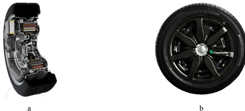
Figure 3.25 – a - In-wheel motor from Schaeffler AG [178], b - Demonstrator of Fraunhofer LBF [153]
