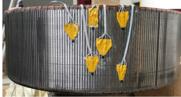
Figure 6.19 – Experimental set-up for the B-field measurement
