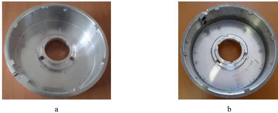
Figure 5.5 – Variants of the stator: standard material variant (a) and hybrid variant (b)
