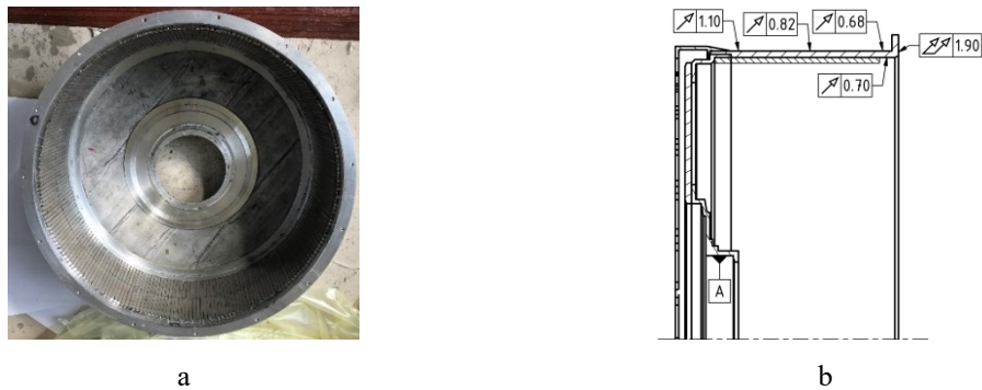
Figure 5.2 – Non-full aluminum foam variant of the rotor (a) and the results of its run-out measurement (b)
