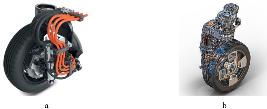
Figure 2.5 – Compact wheel module from: a - Schaeffler [147] and b - Protean Electric [136]
