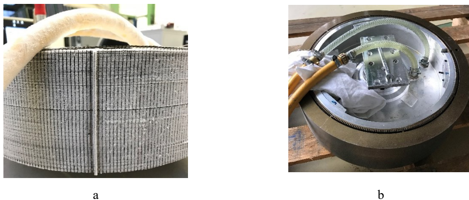
Figure 5.6 – Cooling of the stator by shrinking (a), mounted stator and back iron with additional ring (b)
