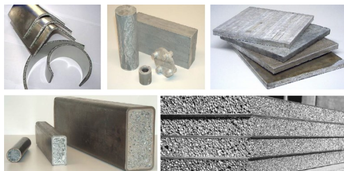
Figure 3.27 – Variety of products based on metal foam sandwich technology [136]
