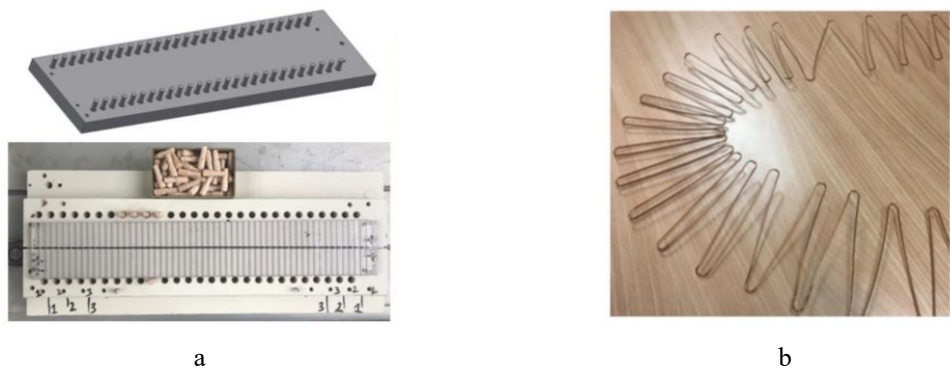
Figure 5.9 – Device for the pre-shaping of the slot windings (a) and bended windings of the slot winding (b)
