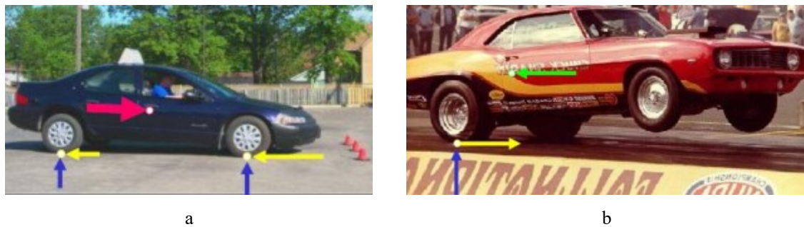
Figure 3.15 – Pitching moment while: a - Braking, b - Accelerating [118]
