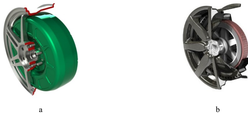
Figure 3.8 – Solutions for torque transferring: a - In-wheel motor from Protean Electric, Inc. [73], b - Demonstrator of Fraunhofer LBF [152]
