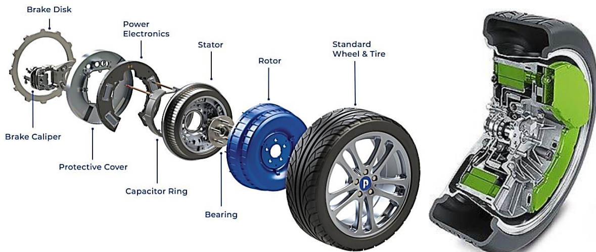
Fig. 2. Protean Electric Pd18 (left) [25] and Schaeffler "E-Wheel Drive" [29] Wheel-Hub Motors.
