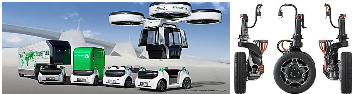
Fig. 4. The Wheel Module (right) and Vehicle Concept Designed for the Future from Schaeffler [29].
