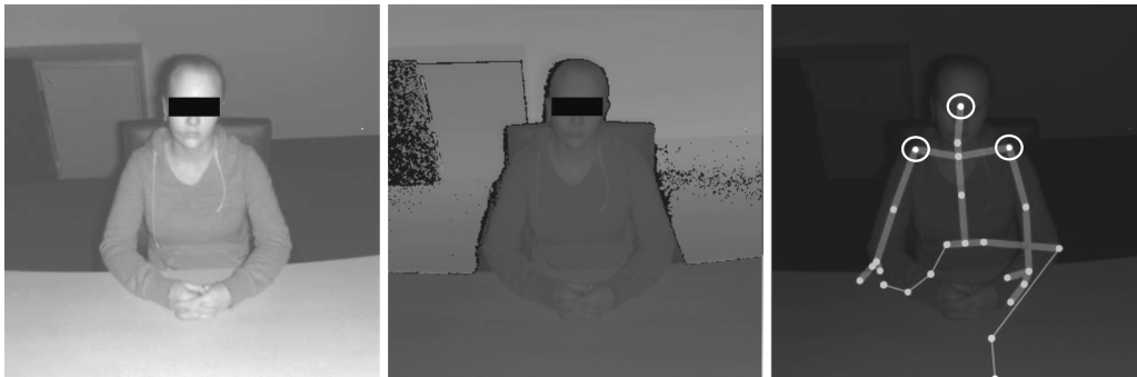
Figure 4.1: A scene from the LMCv2. From left to right: infrared image, depth image, recognised body points (H, LS and RS are encircled).
