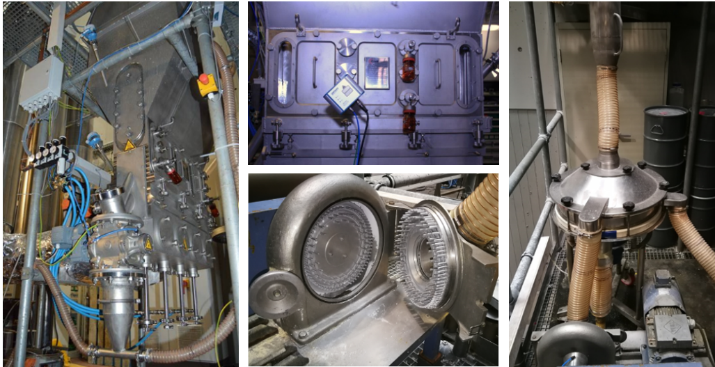
Figure 4.2.: Pictures of the utilized experimental equipment; The pilot-scale plant is located at Hamburg University of Technology: Left: Granulation chamber Procell 25 of Glatt GmbH. Center Top: Granulation chamber equipped with Parsum probe and sampling devise. Center Bottom: Impact mill equipped with pin-mill grinding inlet. Right: Two-deck-tumbler screen and impact mill.
