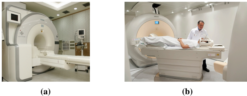
Figure 2.12: Subfigure (a) depicts a Siemens Biograph 3T mMRI scanner [368]. This machine uses a single-gantry design with combined PET and MRI hardware. In contrast, Subfigure (b) shows a Philips Ingenuity TF Whole Body PET/MR system with a multi-gantry design (also called tandem ) [523].
