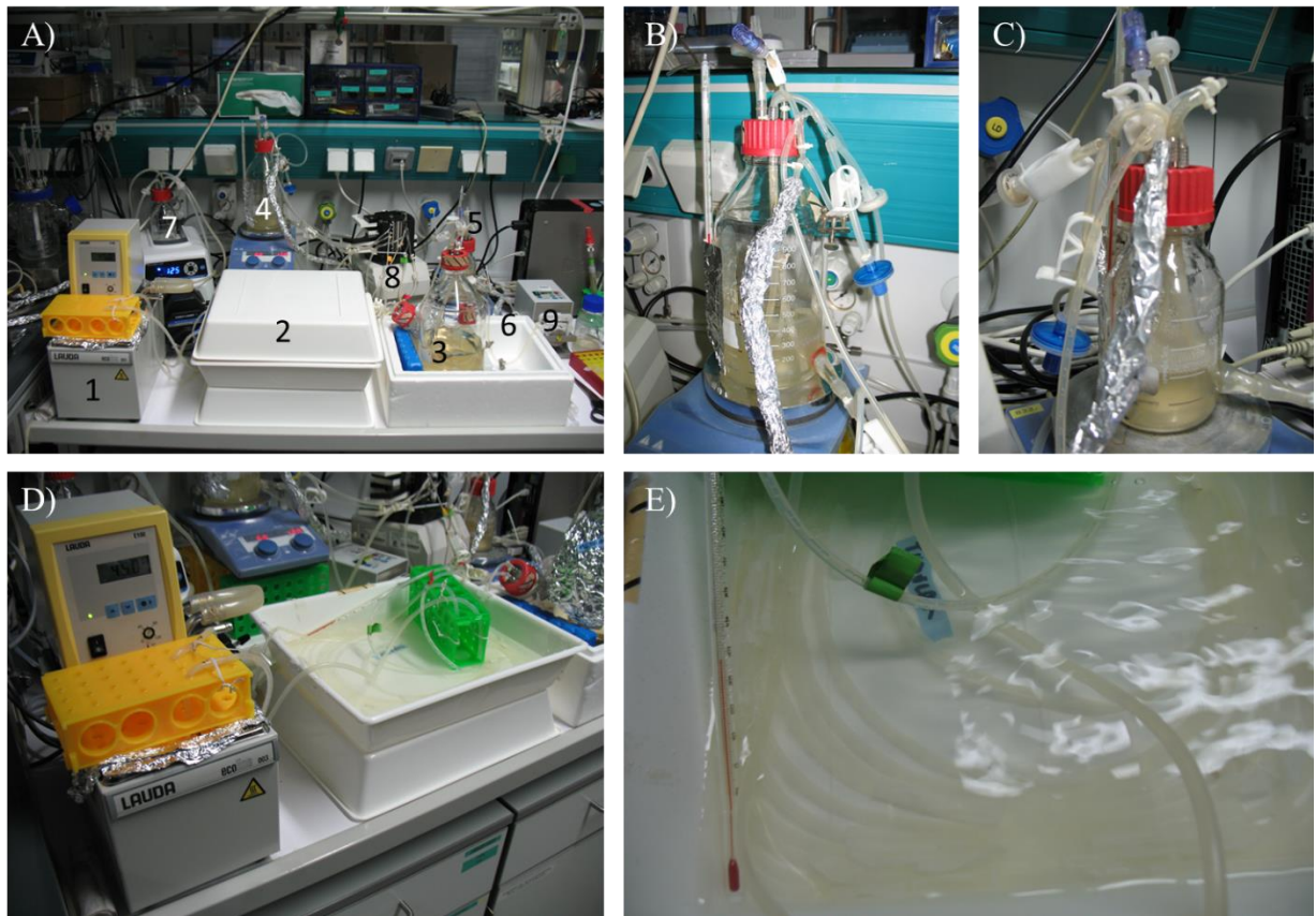
Figure 3. 3. Photograph of the cascade of two CSTRs with recirculation. A) Overview of the bioreactor: Water heating system (1), tubular bioreactor container or PFBR-container (2), stocks of fresh medium (3), cell bioreactor, CB (4), virus bioreactor, VB (5), harvest bottle (6), gas distribution bottle (7), pump 1 (8), pump 2 and 3 (9) . B) 1 L CB for cell growth and with recirculation line to avoid cell sedimentation, covered in alumina foil. C) 250 mL VB for virus propagation and recirculation line to the PFBR covered in alumina. D) Water bath (left) and PFBR-container. E) PFBR in water at 37°C with thermometer.
