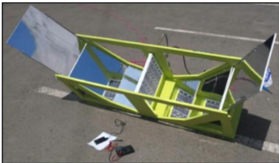
Figure 2: The concept of PVT system with concentrator.
