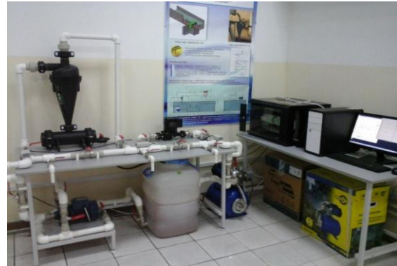
Figure 6: Laboratory installation for studying the parameters of hydroelectric power stations with a hydrocyclone.
