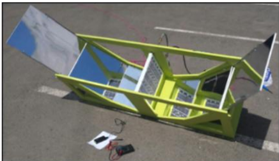
Figure 2: The concept of PVT system with concentrator.
