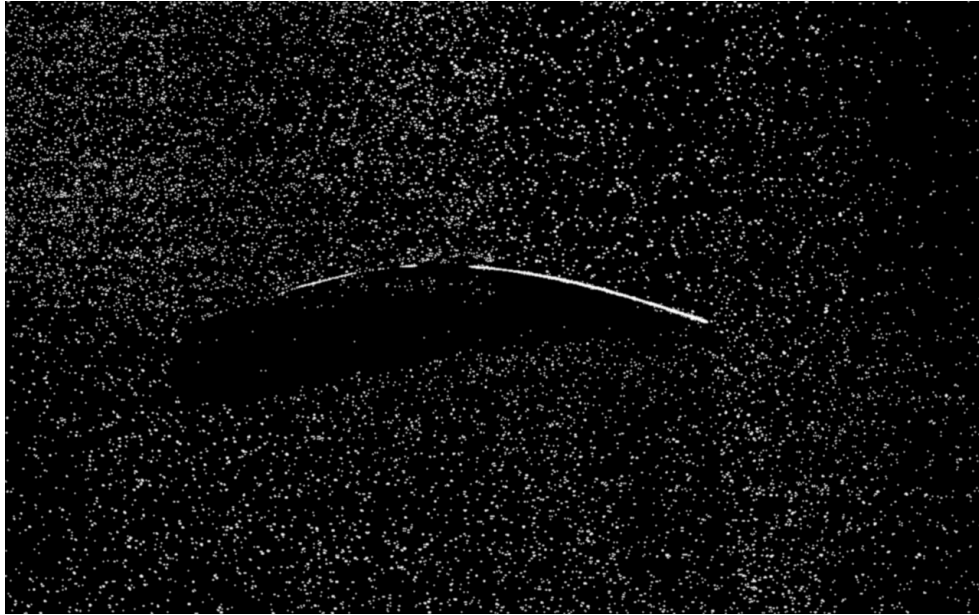
Figure 5.56: A raw image acquired from PIV measurements in the water channel. Particles are visible in white against the black background, with a flexible hydrofoil displayed in the center. The particle density is low due to the particularities of the experimental setup (see sec. 5.4) (particles highlighted for better visibility).
