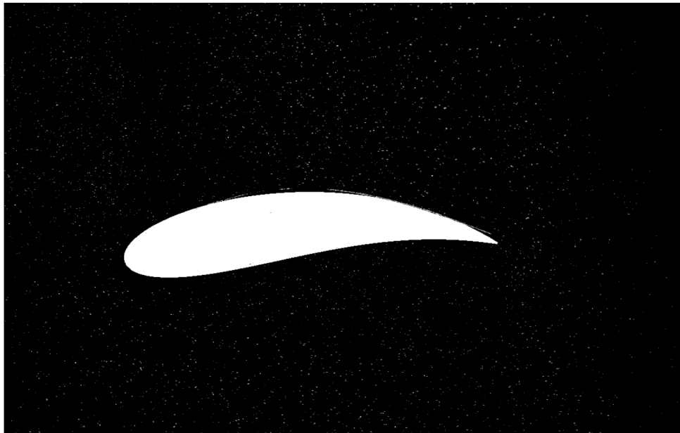
Figure 5.60: The structure retrieved from the segmentation algorithm, embedded in the raw data. The deformed hydrofoil is found with good accuracy. However, because of a phase lag, reflections at the trailing edge become visible in some samples. A video is accessible at the author's website.
