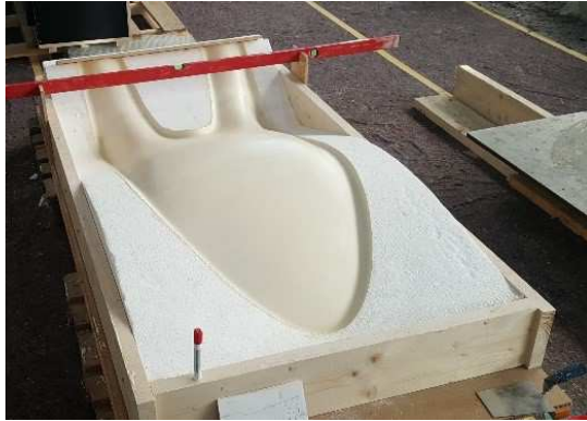
Fig. 30: Surface with Styrofoam filler and measuring of material thickness
