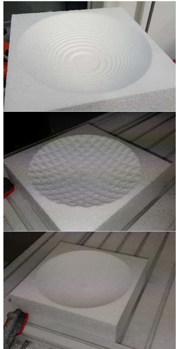
Fig. 10: Surface qualities as a result of different milling strategies
