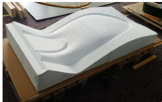
Fig. 29: Assembly of the milled Styrofoam mold parts
