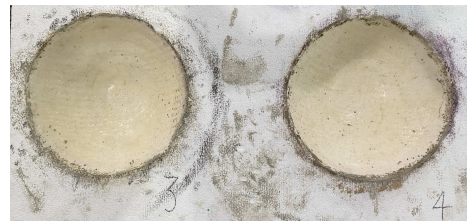
Fig. 6: Molds tested with epoxy resin as surface finish
