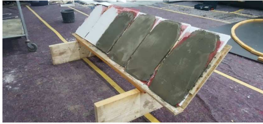
Fig. 9: Hand lamination specimen with different concrete mix ratios
