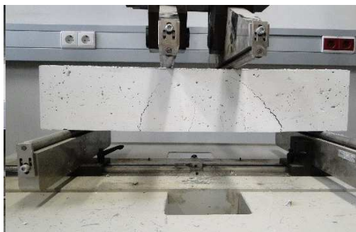
Fig. 5: Four point bending test for textile reinforced concrete
