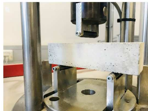
Fig. 1: Dimensions of the sample and support system for Flexural strength
