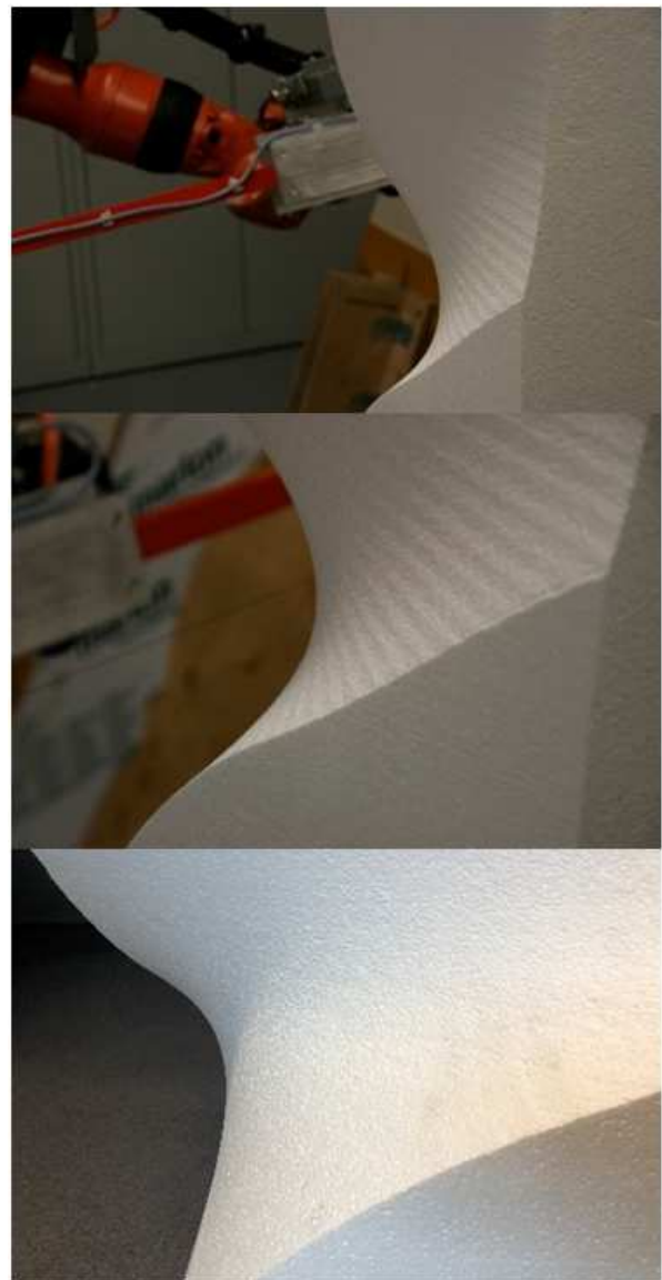
Fig. 11: Surface qualities as a result from hotwire cutting with different cutting speeds
