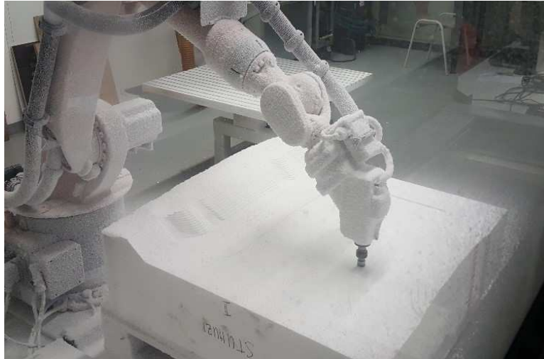
Fig. 22: Robot milling the segments in full scale
