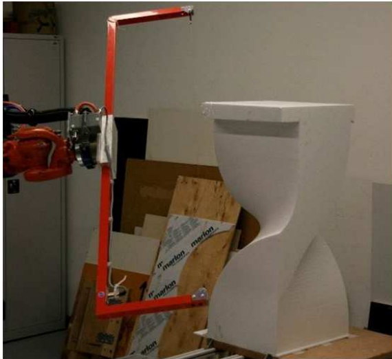
Fig. 18: Robot cutting the prototype in full scale
