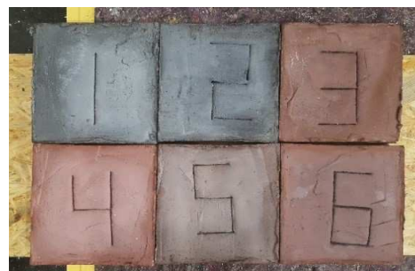
Fig. 8: Concrete blocks with different pigments
