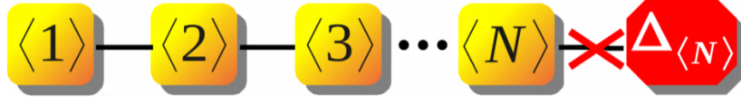
Figure 2.3: Schematic representation of an EV hierarchy. The EV of a certain order connects linearly to the next order that is shown by the black line. The truncation operator \Delta_{\langle N \rangle} is applied by setting the (N + 1) EV to zero. The figure is taken from [Leymann et al., 2014]
