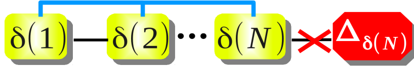
Figure 2.4: Schematic representation of a CF hierarchy. The black line indicates the connection between the first-order CF to the second-order CF and the second-order to the third-order quantity and so on. The blue lines illustrate the production of lower-order CF. The (N + 1) th CF is set to zero by using the truncation operator \Delta_{\delta(N)} . In contrast to Fig. 2.3, the structure of CF hierarchy is nonlinear. The figure is taken from [Leymann et al., 2014].
