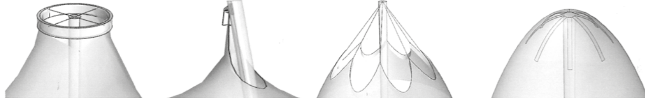
(1) Rigid clamped ring (2) Eye loop (3) Suspended high garland edge (4) Hump
