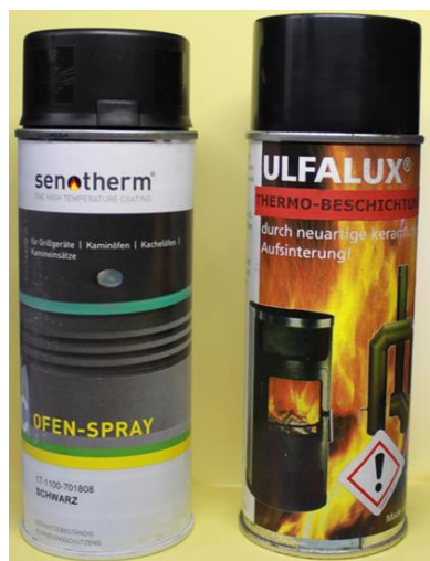
Figure 2.24: Used thermal coatings: Senotherm (left, up to 500 °C); Ulfalux (right, up to 1200 °C)
