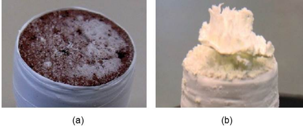
Figure 2.1: NaCl crystals formed at the surface of porous medium: (a) without inhibitors and (b) with inhibitors (adopted from [31]).
