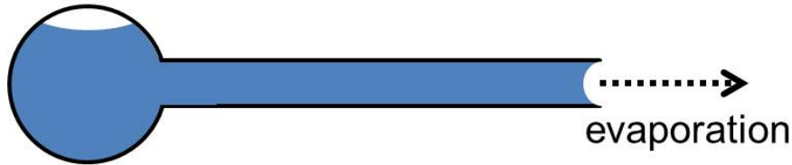
Figure 2.6: Schematic presentation of the first test problem of a capillary connected to a reservoir and open to evaporation.
