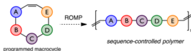
Figure 9: Synthesis of sequence-controlled polymers using ROMP. Figure reproduced from reference 107 with permission from the American Chemical Society.
