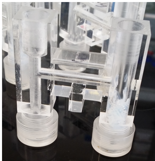
Figure 5.5. – Electro-elution chamber. Gel slices are filled into the broad side of the chamber. The chamber is then filled with electro-elution buffer so that the whole chamber including the bridge is filled to guarantee a current flow.
