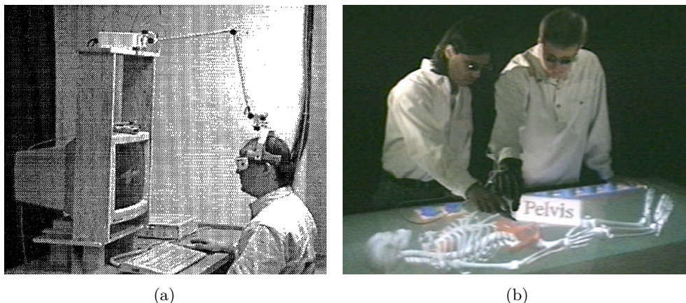
Figure 2.21: In (a), an early semi-immersive fish tank virtual reality system is shown that combines a stereoscopic display with mechanical head tracking [8]. In (b), the responsive workbench is used in a collaborative scenario for anatomy education [2]. Image (a) from Arthur et al. [8] © ACM 1993. Image (b) from Agrawala et al. [2] © ACM 1997.
