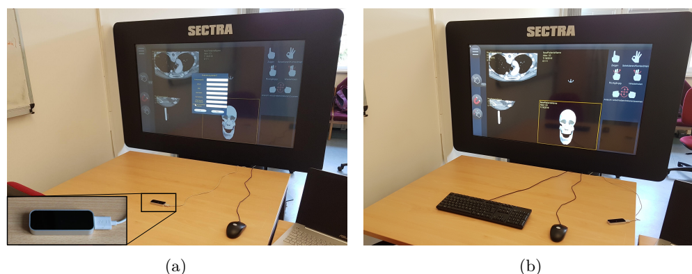
Figure 4.10: The evaluation setup for the gesture-based control (a) and mouse & keyboard control (b). Images were created by Saalfeld et al. [232] and made available in the digital library of the Gesellschaft für Informatik under the Creative Commons BY-SA 4.0 License.
