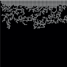
Figure 6-11 Phase distributions from drying with temperature variation from experiment and separate invasion of liquid pores. S = [0.79, 0.4, 0.2] .
