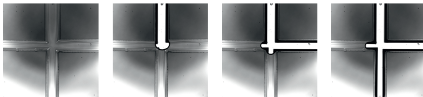
Figure 4-2 Pore scale capillary invasion of a pore junction with 4 adjacent throats. Dry pore space in white, liquid and solid in gray and liquid films confined inside the black zone also in gray.
