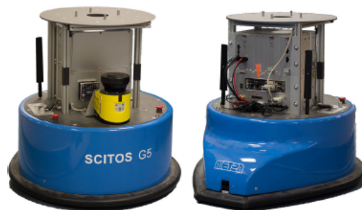
Figure 5.4: Mobile robot platform SCITOS G5 from MetraLabs (Photo: Tony Gieseler [Gie17])
