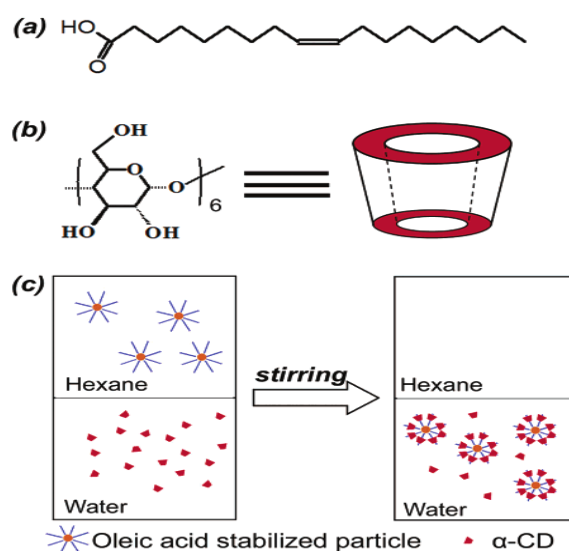
Figure 35: Chemical structure of (a) oleic acid, (b) \alpha -cyclodextrin (CD), and (c) organic to aqueous phase transfer process of oleic acid modified nanoparticles when using \alpha -CD as surface modifying agent [232]
