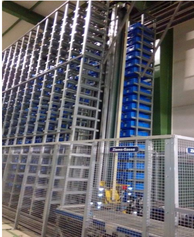
Figure 3.10: Automatic small parts warehouse (ASPW) at the Institute (ILM).
