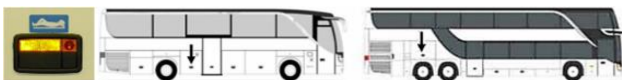
Figure 12 – Location of Driver's Sleeping Room in High Deckers and in Double Deckers [38]
