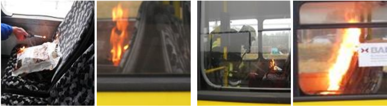
Figure 52 – Sources of Smoke Scenario III (both left) and Smoke Scenario IV (both right)
