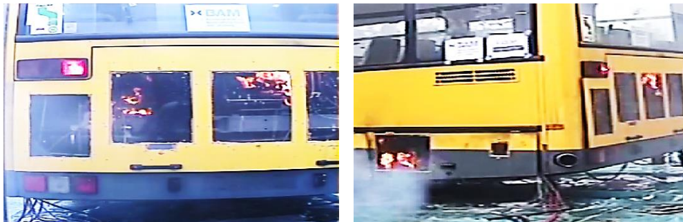
Figure 44 – Fire Scenario I of Engine Compartment Fire Tests
