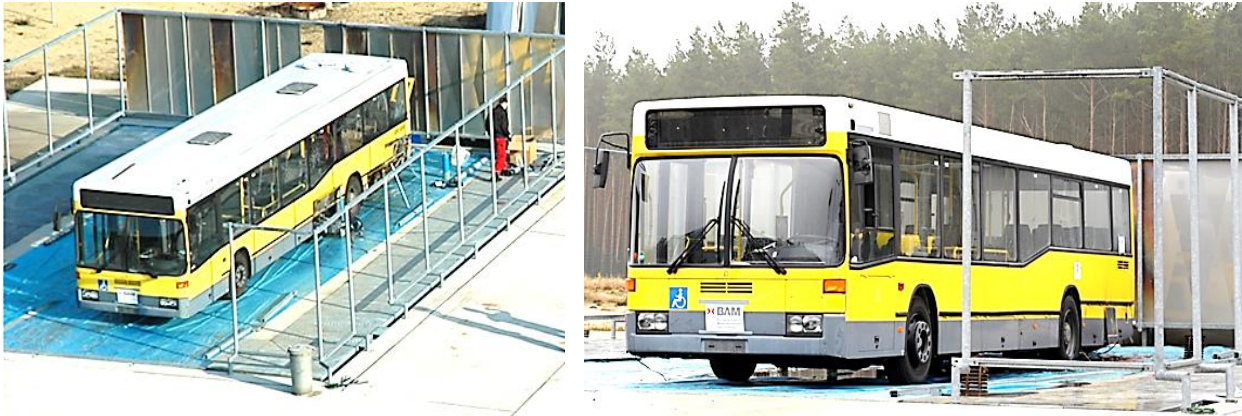
Figure 39 – Test Bus at Fire Test Stand of BAM
