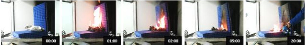
Figure 33 – Train Passenger Seat compliant to EN 45545-2 in Calorimeter Test
