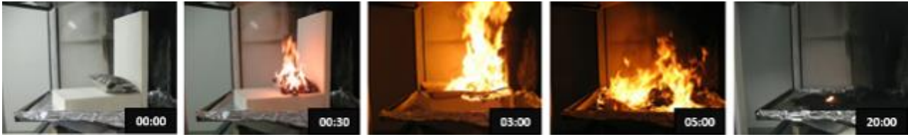
Figure 30 – Coach Passenger Seat compliant to UNECE R 118 in Calorimeter Test
