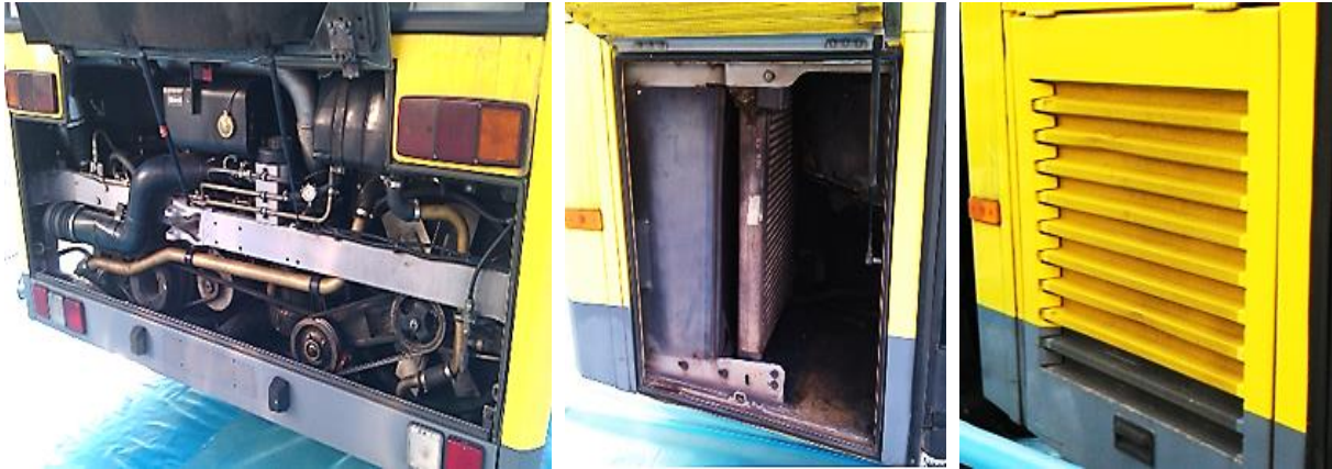
Figure 41 – Outer Maintenance Flaps of Engine Compartment at Test Bus
