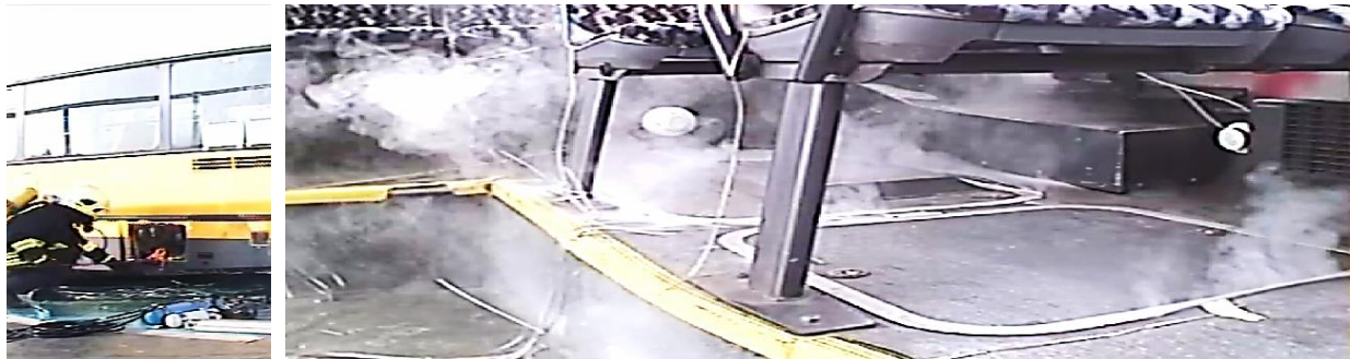
Figure 48 – Ignition and Smoke Penetration into Passenger Cabin in Fire Test 05
