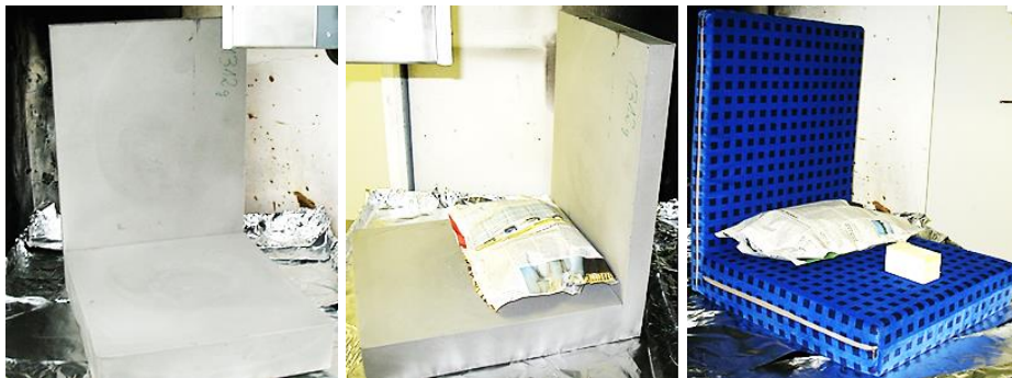
Figure 32 – Train Passenger Seat compliant to EN 45545-2 prior to testing
