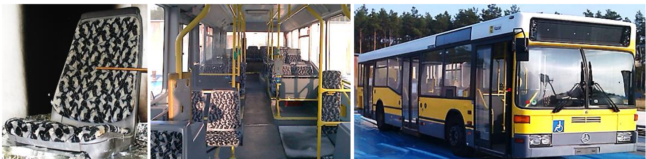
Figure 26 – Bus Passenger Seat compliant to DIN 5510 tested and Donor Bus
