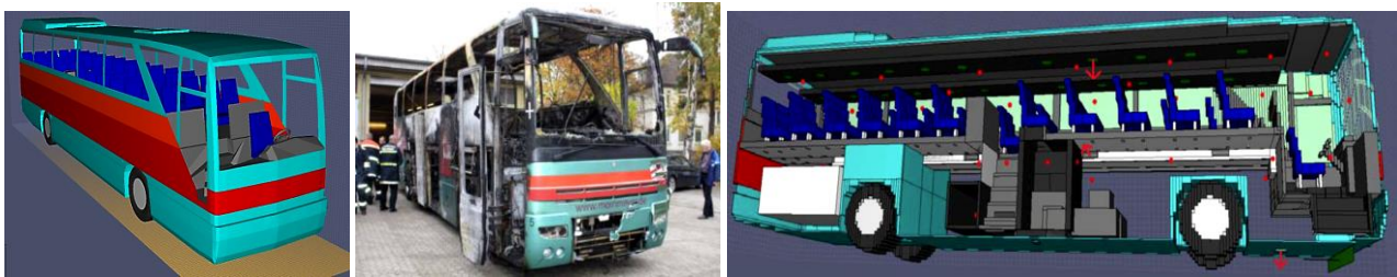
Figure 62 – Hanover Bus Fire Model [69] and Wreck of Hanover Bus Fire [70, 71]
