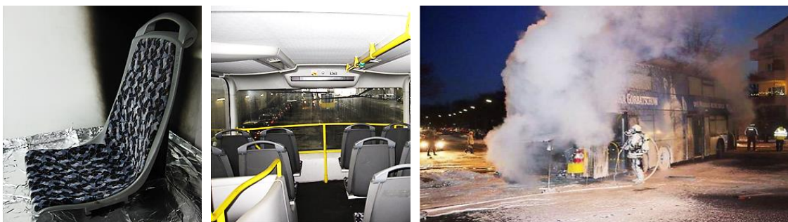
Figure 23 – Bus Passenger Seat compliant to UNECE R 118 tested and the Donor Bus [58]
