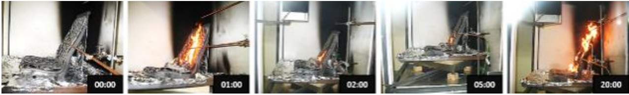
Figure 27 – Bus Passenger Seat compliant to DIN 5510 in Calorimeter Test
