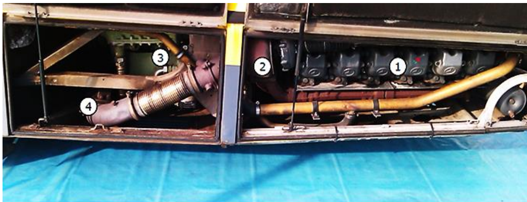
1 Engine block 3 Automatic gearbox 2 Turbocharger 4 Manifold
