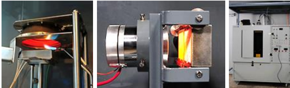
Figure 19 – Smoke Density Chamber used in Laboratory at BAM [50]
