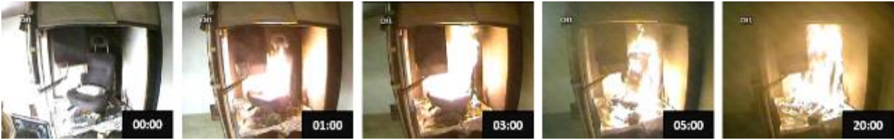
Figure 36 – Car Driver Seat compliant to ISO 3795 in Calorimeter Test
