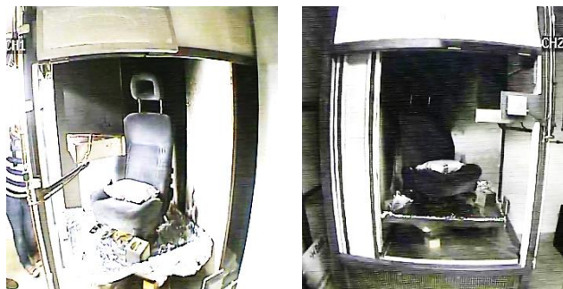
Figure 35 – Car Driver Seat compliant to ISO 3795 prior to testing
