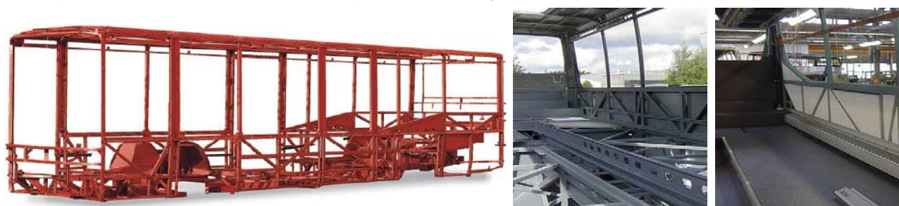
Figure 7 – Typical Base Frame of Buses [38]
