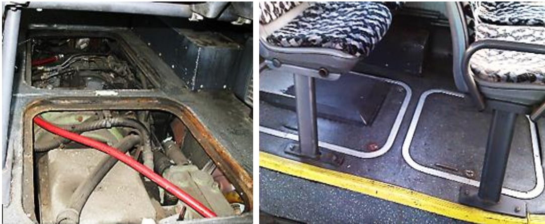
Figure 42 – Inner Maintenance Flaps of Engine Compartment in Passenger Cabin
