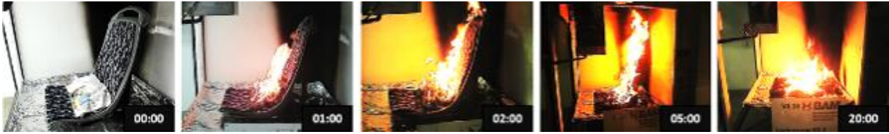
Figure 24 – Bus Passenger Seat compliant to UNECE R 118 in Calorimeter Test
