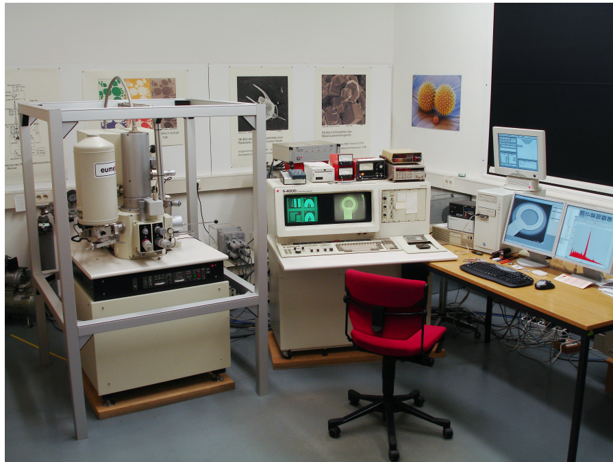
Figure 4.5: The Hitachi S-4000 SEM at the ZELMI. It has been used to take the images used for this thesis. On the left, the microscope itself can be seen. It stands on a special table to reduce vibrations, which could lead to image artifacts, and is surrounded by a frame to reduce the impact of electromagnetic radiation on the images. In the center, there is the console used to control the microscope. On the right, one can see the computer used to digitally save the images. Picture by ZELMI.
