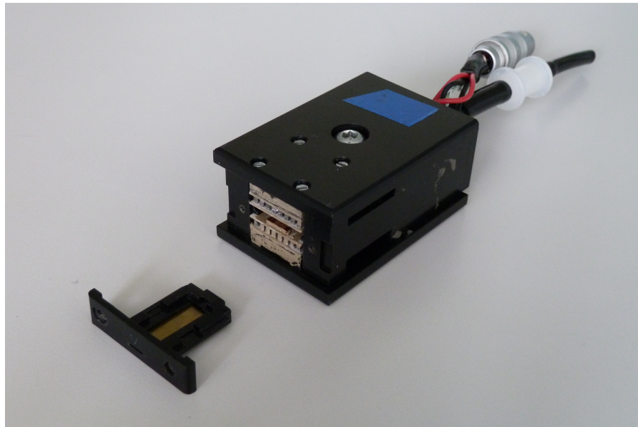
Figure 4.1: The thermal precipitator used by the BAuA. At the front, the tray which holds the silicon substrate onto which the particles are deposited can be seen. In the back, there is the cable and the tube which connect to the power source and the air pump, respectively. Picture by BAuA.
