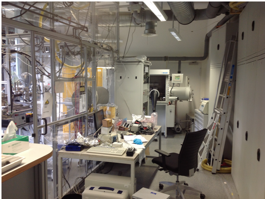
Figure 2.3: Picture of ZnO nanoparticle production on a laboratory scale. On the left, the enclosure which is housing the production apparatus is visible. On the far left, the enclosure has an opening, which can be closed by a sliding door. Picture by BAuA.
