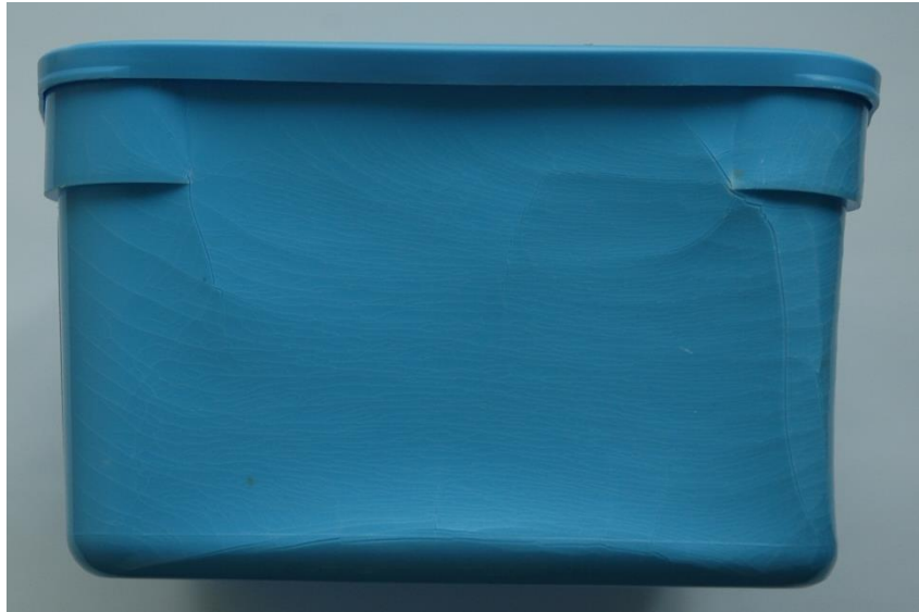
Fig. 12: PP-Box after three year indoor weathering (radiation from sunlight through a window pane)
