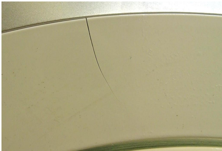
Fig. 13: Crack in a PP-component induced by aggressive solvent
