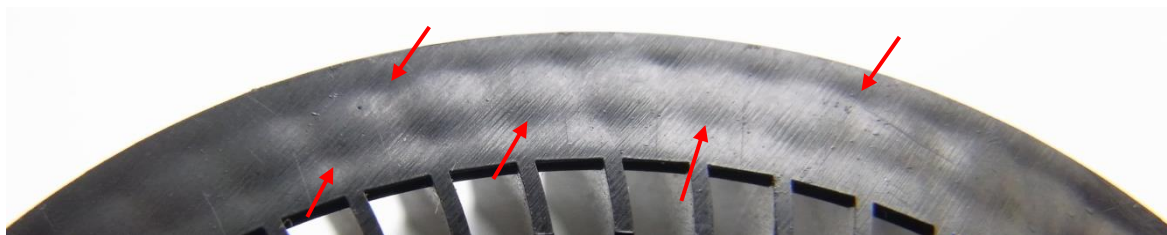
Fig. 3: Sink marks on an injection molded PC/ABS-component in a region of large wall thickness (stiffening ribs)
