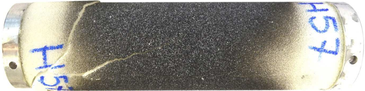
Fig. 1: Internal pressure test on the foam specimens made of ROHACELL®110 IG without protective layer inside the specimen with \varnothing_{\text{outer}} 58 mm, \varnothing_{\text{internal}} 40 mm and length 200 mm.
