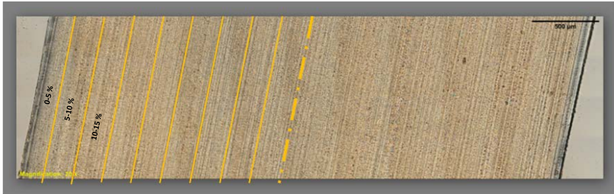
Figure 3. Polarized light microscopy image of injection molded cross section, before sectioning samples for FDSC.
