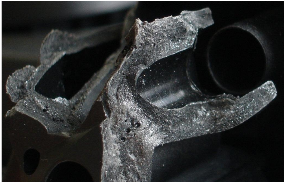
Fig 8: Fracture surface of a mineral filled PA6-component with gas bubbles
