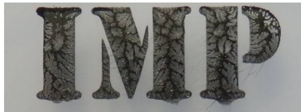
Figure 2: Influence of the melt temperature on ink transfer during injection molding ( T_{\text{melt}} = 280^{\circ}\text{C} , T_{\text{mold}} = 30^{\circ}\text{C} , p = 350 \text{ bar} )
