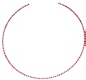
1- Subdivide curve into vertical frames
