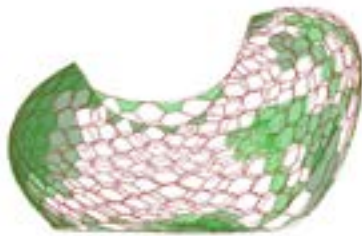
9- Run simulation in Kangaroo to planar each hexagon
