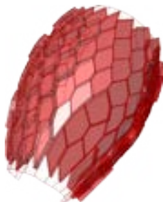
3- Extrude Hexagons with random values in direction of surface norm
