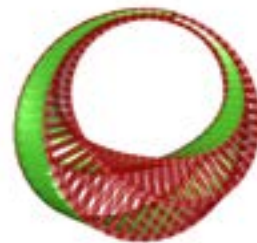
6-Create 2 surfaces by lofting the edges' curves
