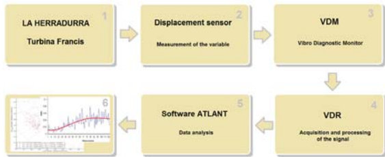
Figure 3: Measurement chain of vibration analysis system.
