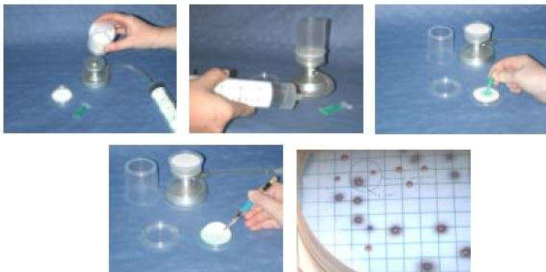
Abb.1 : Membranfiltration [4]
