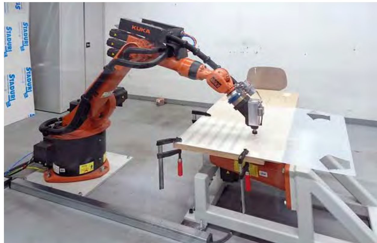
Milling of polymer sheets
