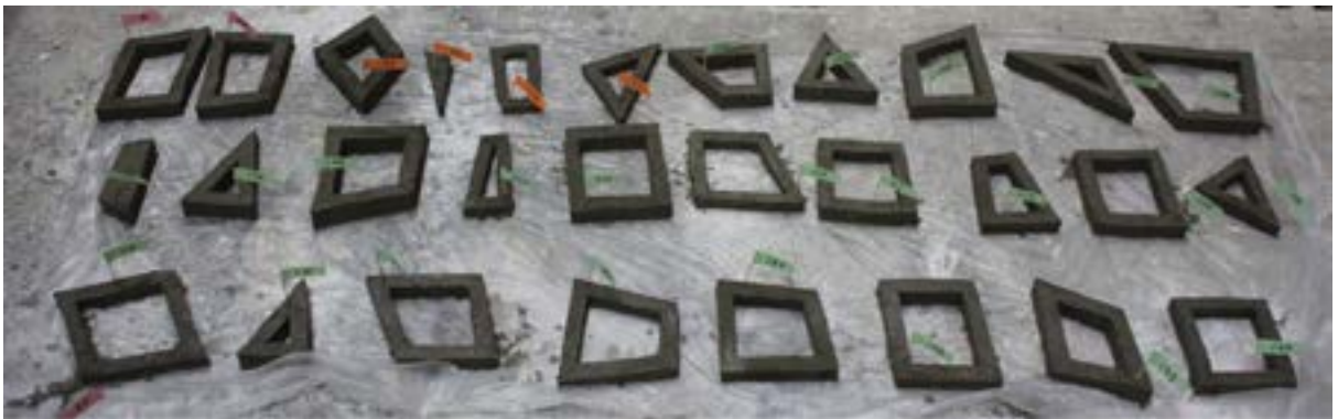
Fig. 09: Custom shaped blocks, formed with the 'positive casting' method, Smart Masonry, Dmytro Zhuikov & Arina Agieeva, Studio Krastev, DIA, 2015.
