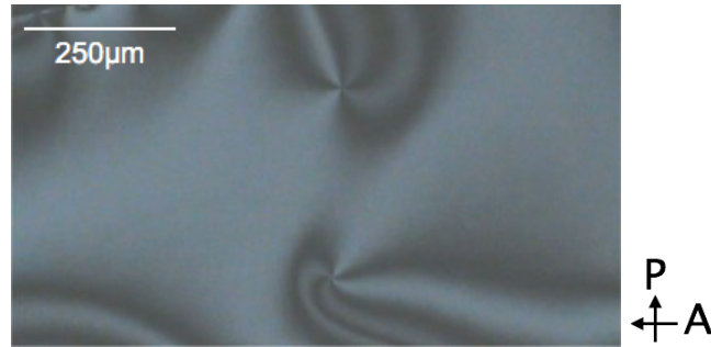
FIGURE 2.13: Reflective microscopy image of a defect structure in a SmC film between crossed polarizers.
