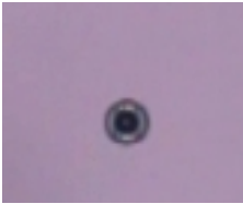
FIGURE 4.4: Reflective microscopy image of an embedded droplet in a FSF of M5N . The picture was taken about 12s after impact with a magnification of 3.3 \mu\text{m}/\text{Pix} . It reveals the meniscus around the droplet.
