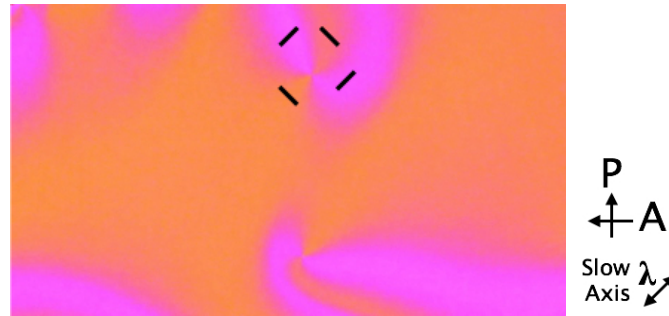
FIGURE 2.15: Reflective microscopy image of the defect structure in figure ???. The SmC film is illuminated between crossed polarizers with a \lambda -wave plate. Dashes indicate the orientation of the SmC director around the topological defect.
