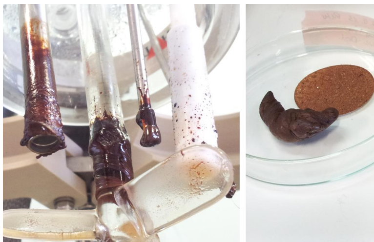
Figure 56: Lignin incrustations and lumps formed by the soft or liquid lignin during the process.
