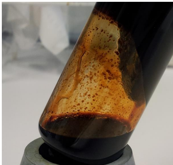
Figure 42: The photograph shows a glass vial that was turned upside-down a few seconds before taking the photo. It contains a sticky solvated lignin-rich phase that slowly flows down and a black liquid solvent-rich phase beneath that already rinsed down the vial.
