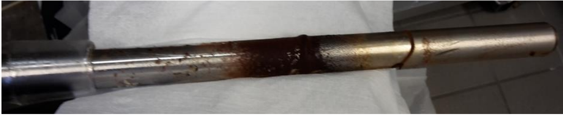
Figure 65: Lignin incrustations on the FBRM ® probe formed by foaming of the boiling lignin dispersion.
