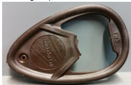
Figure 4: Bottle opener consisting of an experimental lignin-cellulose composite manufactured by injection molding in a joint project of Fraunhofer CBP, Tecnar GmbH, FWS GmbH and MPI Magdeburg.
