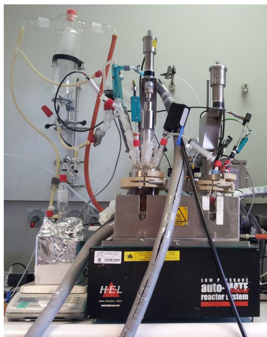
Figure 22: Left: Process flow chart of the experimental setup for lignin precipitation in a batch reactor. Right: Photograph of the experimental setup for lignin precipitation in the batch reactor (300 ml).
