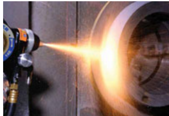
(b) Coating process using thermal spraying technique [2].
