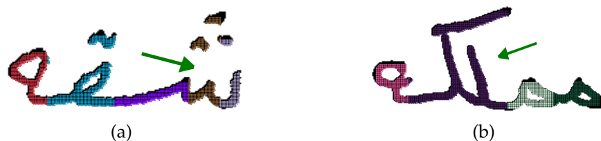
FIG. 6.7. Over and Under segmentation errors: (a) Over segmentation problem where letter ش is erroneously segmented into two parts, (b) under segmentation problem with two letters ل and ك merged into one.
