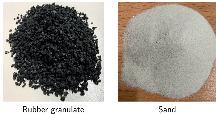
Figure 7.4: Materials used to investigate particle damper behavior under dynamic loading and temperature fluctuations.
