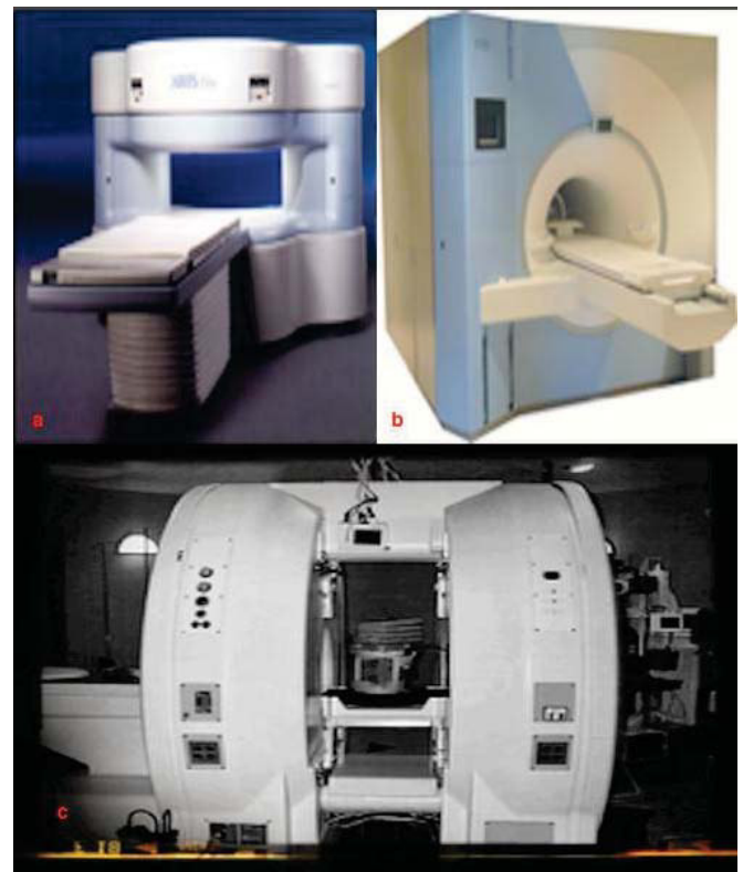
Fig 2: Different MR systems. a) Open bore b) Closed bore c) Double Donut configuration
