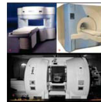
Different MR systems. a) Open bore b) Closed bore c) Double Donut configuration
