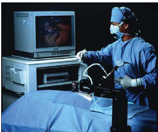
Figure 1 : Aesop is a voice -activated robotic arm that holds the camera and endoscope assembly for the surgeon during an endoscopic procedure.
