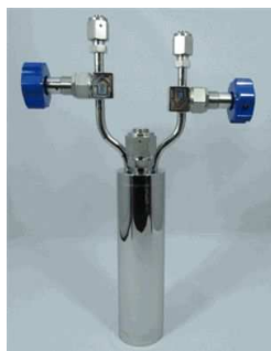
Figure 2.16: Vertical electropolished stainless steel bubbler [78]
