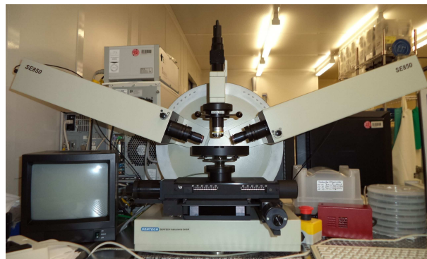
(e) Goniometer, sample stage, optical camera, polarizer, analyzer and detector
