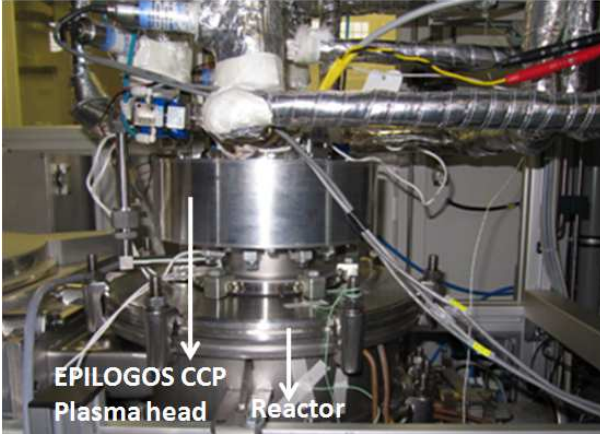
(a) 'HFO' PALD system (single wafer reactor) with 'EPILOGOS' CCP plasma source
