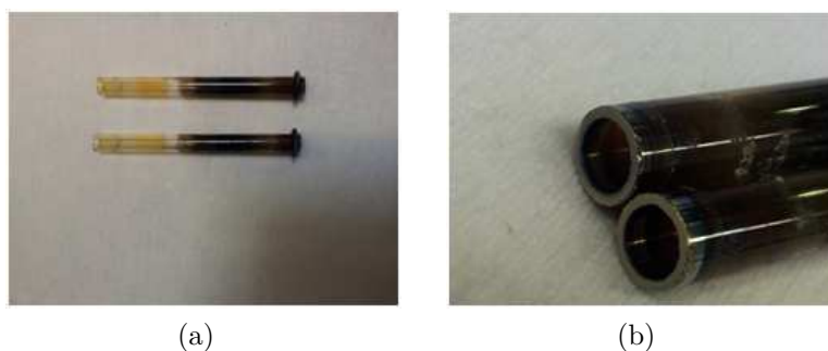
Figure 5.10: Coatings inside the dual plasma tubes after several ALD processes
