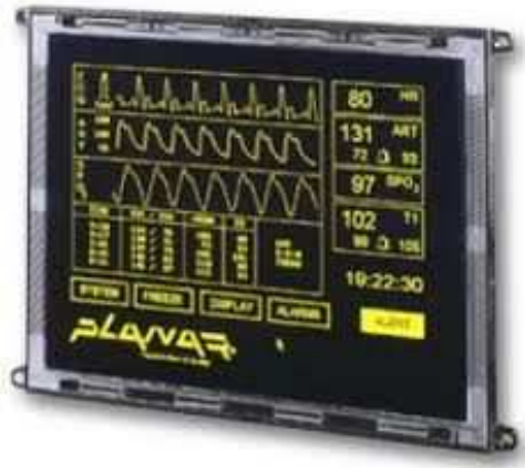
Figure 2.10: Thin film electroluminescence display [66]
